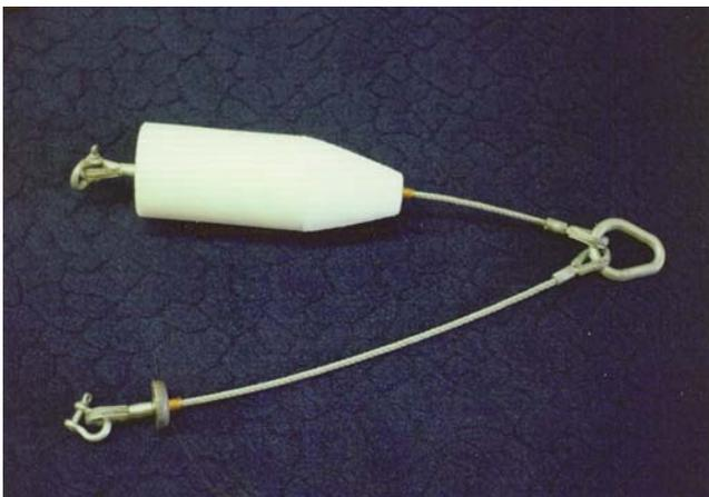
**TOW BRIDLE ASSEMBLY:** This system provides a stable two-point tow load and can be used with any boom which has a built in tow assembly or either of the Tow Adapter systems shown above. It includes a pear link, galvanized or stainless steel cables, float, ballast, galvanized steel shackles and is sized for service of the boom it supports.
